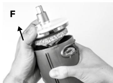
**Pictures E & F:** Holding the flange as shown in your left hand, turn the inner body to the right until it stops. Take the flange away from the inner body in your left hand you are holding the rotor (rotating stone), in your right the stator.
