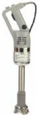
ROBOT COUPE CMP IMMERSION BLENDER Shaft length: 10". Volts: 120. Hertz: 60. Amps: 1.1. Watts: 310. Single phase. RPM: 5,000 to 10,000 (variable). ETL (European) sanitation and electrical listed. P313
